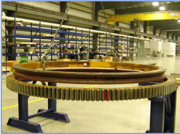
Figure 1 - Crossed-roller slewing bearing with external gear teeth: Rings, rollers and spacers received for repair.
