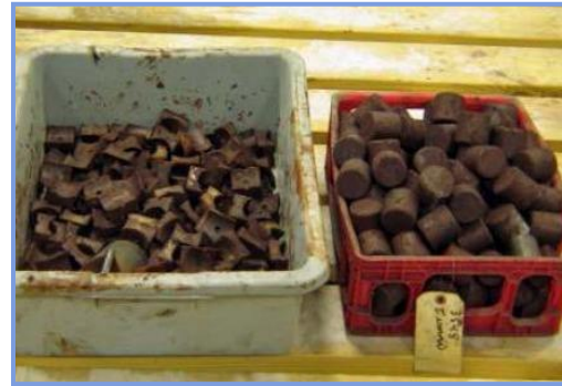
Figure 1 - Crossed-roller slewing bearing with external gear teeth: Rings, rollers and spacers received for repair.
