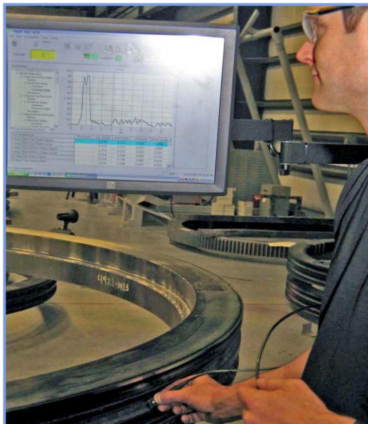
Figure 2 - Hardening depth data measurement with ultrasound spectrometers.
